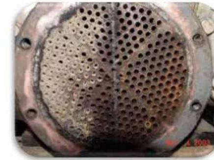
De-scaling of industrial equipment (boilers, heat exchangers, etc) is probably necessary during normal annual maintenance, to improve performance and effectiveness of heat transfer.
